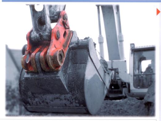
A-Lock mechanical - quick change of attachments without hydraulic supply
