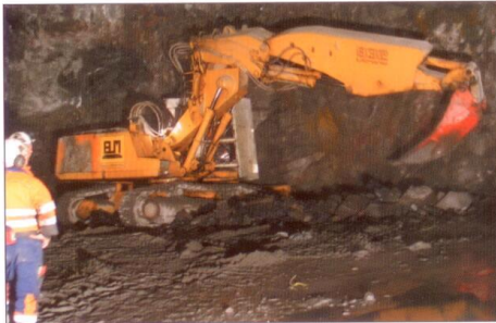
Rock ripper XHD for hard application, made from WHD 450 special wear steel, with Esco ripper-tooth
